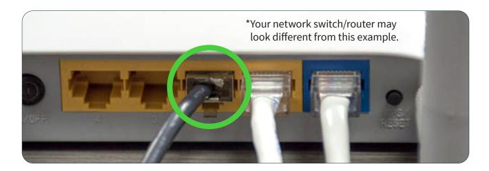
**2B)** Connect Lane/5000 power supply to 120V power outlet and to the back of the Lane/5000 Ethernet cable. *Note: Lane/5000 will turn on once connected to power.*
